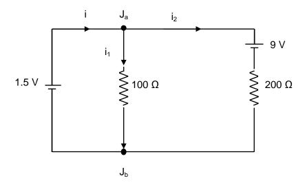
Use the arbitrarily decided directions of i,  $i_1$  and  $i_2$  to treat the circuit as 2 loops joined at junctions  $J_a$  and  $J_b$ . Now use Kirchoff's laws to find the values of the currents i,  $i_1$  and  $i_2$ .
