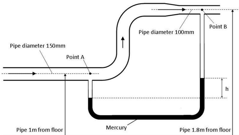
The flow of water through the pipe is  $0.1\text{m}^3/\text{s}$ . Using Bernoulli's formula, calculate the difference in pressure between points A and B, as would be indicated on the mercury column manometer. Show all calculations and any formulae used. Give your answer in millimetres-head. (**Note:** The density of sea water is  $1025\text{kg}/\text{m}^3$  and the density of mercury is  $13,600\text{kg}/\text{m}^3$ .) (10 marks)
