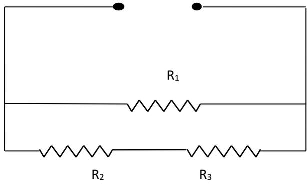
Three resistors are placed in an electrical circuit with a  $230V_p$  (peak voltage) supply as shown in the figure above. Resistor 1 has an average power rating of  $2.5kW$ , resistor 2 has a resistance of  $21.26\Omega$ , and resistor 3 has an average power rating of  $4kW$ . The total peak current flowing in the circuit is  $15A$ . Consider only pure resistance in the circuit, ignoring any reactance.
