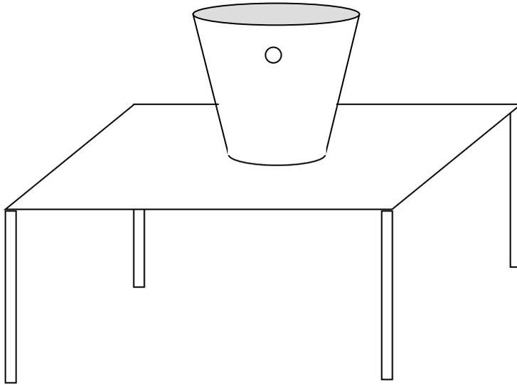
Refer to the diagram above. A plastic container, 60cm high and open at the top, is filled with foam concentrate and placed on top of a table which is 1.3m from the floor. The container has a top diameter of 30cm and a bottom diameter of 15cm. A circular hole of 1.5cm diameter is made in the side of the container such that its centre is 20cm from the top. (Density of foam concentrate =  $850\text{kgm}^{-3}$ )
