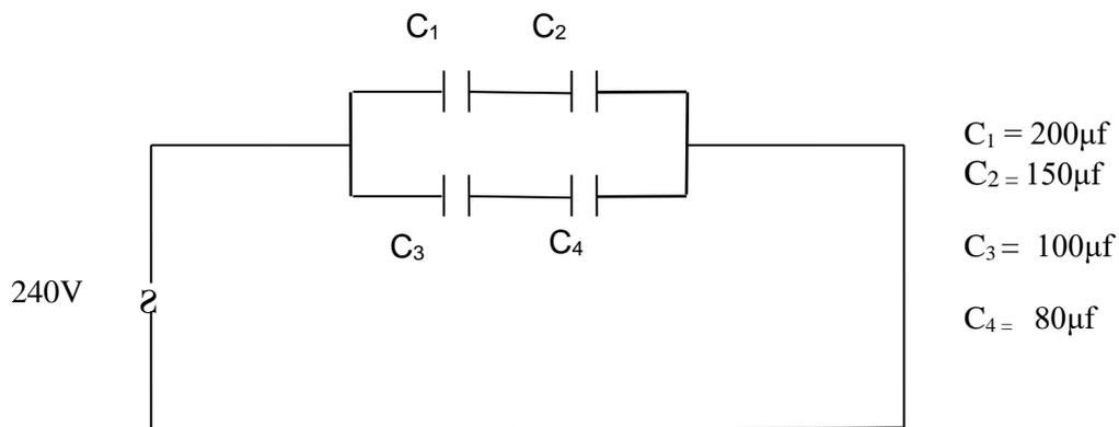
i) If the supply voltage is at 40Hz, calculate the overall capacitance for the circuit. (7 marks)
